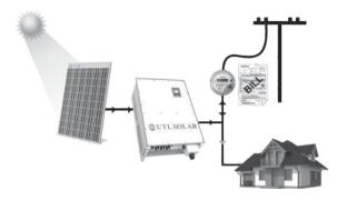
On-grid solar is used to save on electricity bills because it does not have any battery to store solar energy. In an on-grid solar system, the solar inverter is directly connected to the electricity supply. The electricity generated is used by the customer, and the remaining units are deducted from the electricity bill. This process of offsetting electricity usage is called net metering. Across India, net metering is used exclusively for residential on-grid solar systems.
