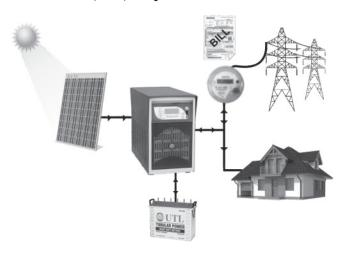
Hybrid solar is a combination of off-grid and on-grid solar systems. It includes batteries to provide backup during power cuts and also has the provision to send excess solar energy back to the grid when it is not being utilized.
