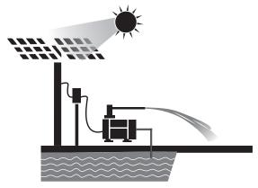
Agricultural pumps used for irrigation are now being powered by solar energy. Solar agricultural pumps do not include batteries. The solar energy generated by solar panels is converted through a motor pump controller to run the water pump. The more sunlight falls on the solar panels, the more solar energy is generated, and the faster the pump can draw
