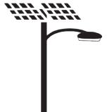
You must have seen street light solar systems. Today, the lights on electric poles are often LED lights powered by solar energy. Small solar panels and batteries are installed alongside the LED lights to run them on both solar energy and electricity. This is known as a street light solar system.
