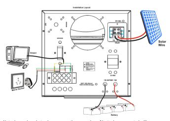
Note: Image is only to show connections, number of batteries connected will be according to the rating of the system.
