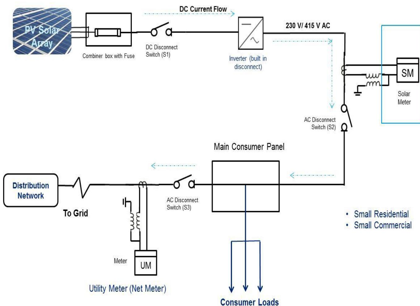
The utility meter (Net-meter) has to be bi-directional meter to register both import grid electricity amount as well as export solar electricity amount.
