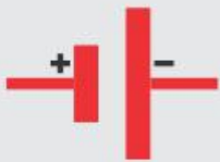
DC Power Supply
